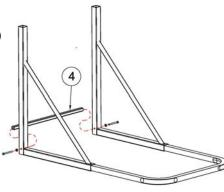
3) Slide upper frame assembly (part 7) into the two side frame assemblies.
