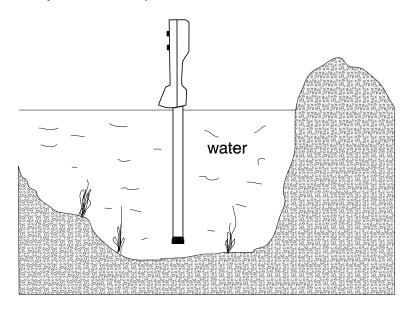
Hold the locator in a vertical position while searching to produce the best results.
