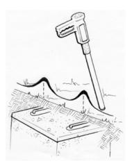
Well Casings are long and produce a strong magnetic field making them easy to locate. Signal response will be very much like that of a manhole cover. Strong at the outer edges with possibly two peaks as you sweep across the casing.
