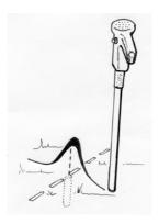
When you are above the target, sweep in an "X" pattern as shown above. As you sweep, note where the signal peaks or is most shrill. Adjust your "X" pattern sweep until the peak from each sweep direction occurs in the same spot. This will help you to find the center of the target object.
