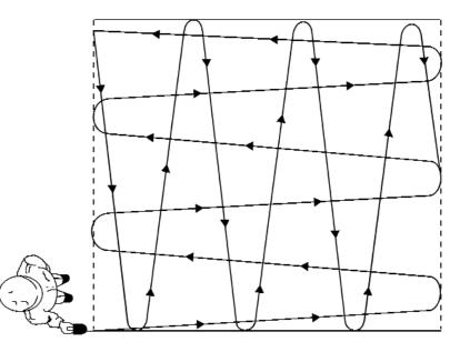
Walk the grid again using the Passive Power. You should now have identified and marked any continuous metal pipe and/or cables, and properly installed tracer wire on plastic/vinyl/PVC pipe within the area.
