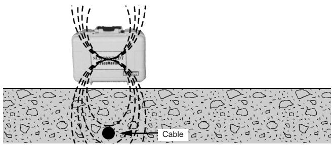
Place the Transmitter on the ground over the cable to be located. The Transmitter arrow should be in line with the cable path, as shown above. Turn the Transmitter on and select
