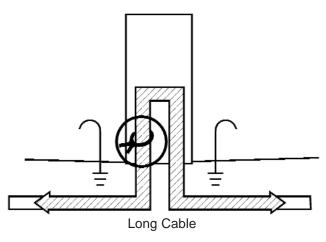
Several cables grounded at a common point present no problem for the Inductive Clamp method. Even though signal is coupled into each cable, the cable with the Clamp is clearly identifiable because it has the strongest signal.
