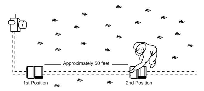
Applying Signal to Power Cables: Inductive Clamp Method
