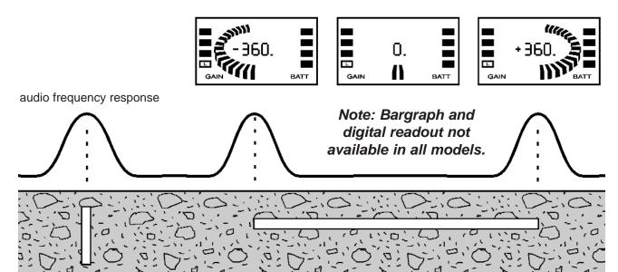
When the Receiver is positioned directly over a vertical pipe, the audio and digital indications will peak. The expanding bar graph and digital readout may be either a positive or negative. The audio response, bar graph, and digital indications peak over each end of a horizontal pipe. One end is positive the other is negative. This will help to distinguish between two vertical pipes or one horizontal pipe. Usually two vertical pipes buried in close proximity will produce similar polarities.
