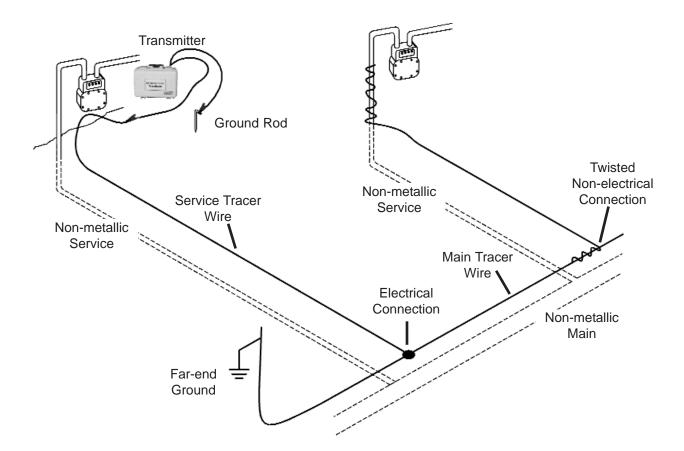
Apply Signal to Pipe: Inductive Clamp Method
