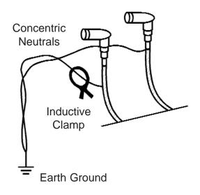
Applying Signal to Secondary Cables To locate secondary cables, the easiest access to the neutral is at the meter box. There are several ways to put signal on the neutral. If the riser pipe is nonmetallic (usually PVC), clamp the Inductive Clamp around the pipe. The jaws of the clamp must fully close for signal transmission. This may be impossible if the riser is flush with the mounting structure or bigger than your clamp.
