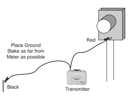
technique is fast since you do not have to open the transformer, or break the meter seal. Select the lowest frequency (575 Hz); it does not couple to other grounded cables as easily as a higher one, but will place equal signals on telephone and CATV cables if common bonding is used.
