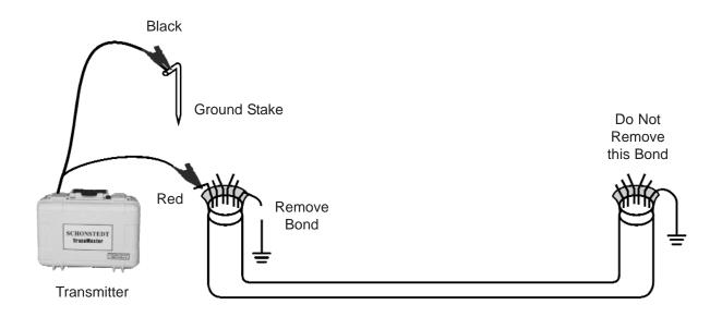
The Conductive method requires access to the cable shield. Disconnect the shield bond at the near-end where the Transmitter is connected. Do not disconnect the far-end shield bond since this supplies a far end ground.
