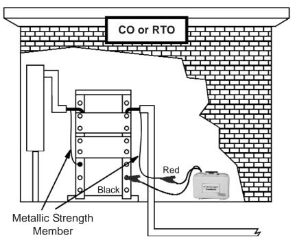
Connect the Conductive connectors to the metal strength member and to the frame or rack ground point.
