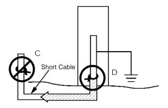
Normally, do not use the clamp on a cable that has the shield ungrounded at both ends. If the cable is long, remove the bonding and signal goes both ways as shown. You must use the highest frequency to increase the signal leakage since there are no grounds
