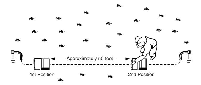
If the Receiver has trouble picking up the cable path, switch to a higher frequency.
