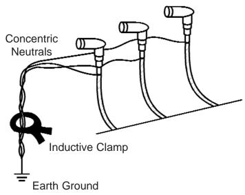
It is important *not* to place the clamp around one of the individual primary cables. Not only is this dangerous, but the cables are buried in the same trench, causing a canceling effect as signal goes one way on one cable and the opposite way on the other.
