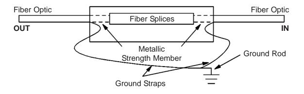
Maximum tracing signal is obtained by disconnecting the bonding strap(s) from the ground point before attaching the Transmitter, but local practice may not allow this. In this case, the signal splits between the incoming cable, outgoing cable, and the ground point, thus reducing the tracing range.
