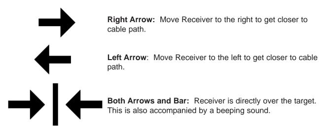
When all three arrow elements are OFF, the signal strength is not adequate to make a directional determination. Keep searching based on the signal strength indication (you may need to increase the gain) and the audio feedback, until one of the arrows comes ON. **Directional indication is not available at 455 kHz.**
