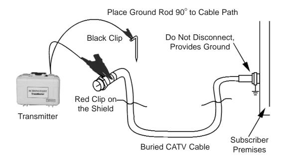
Connect the Conductive connectors to the cable shield and to the ground stake. Connect Red to the shield and black to the stake.
