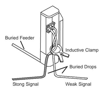
After applying the transmitter signal, walk 10 to 25 feet away from the pedestal. Hold the Receiver so that the display end of the handle points directly to the pedestal. Start walking in a circle around the pedestal with the Receiver always pointing toward the pedestal.
