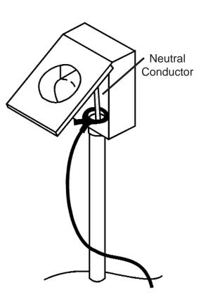
Some meters may have an external ground wire from the meter box to an earth ground. Clamp around the wire as shown. This puts signal on the neutral since the ground wire is connected to the neutral in the meter box. Make sure you place the Inductive Clamp above other utilities that may be grounded at the ground rod, or signal will be applied to them also.
