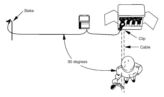
Use the low frequency (575 Hz) so that signal will not couple to other grounded cables. This frequency will travel farthest down the cable.
