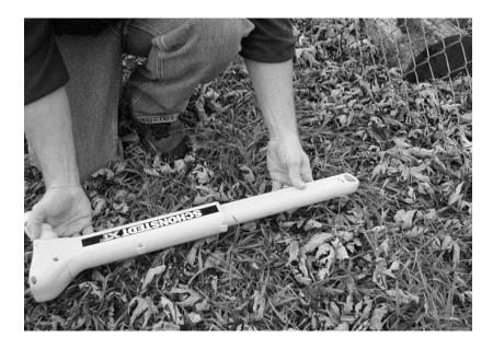
Listen for an abrupt drop in the signal (as shown by the small null in the illustration below) that will occur when the lower sensor, located a few inches from the end of the locator, is directly over the target. Any variation from this position will produce an abrupt rise in the frequency of the signal.
