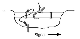
When you use the Inductive Clamp to apply signal to a metallic service line at a gas meter, always ground the valve. This provides good return for signal. Otherwise, the insulating coupling above the valve isolates the returning signal from ground and may make locating the service line difficult.
