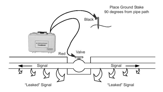
Conductive Method on Tracer Wires
