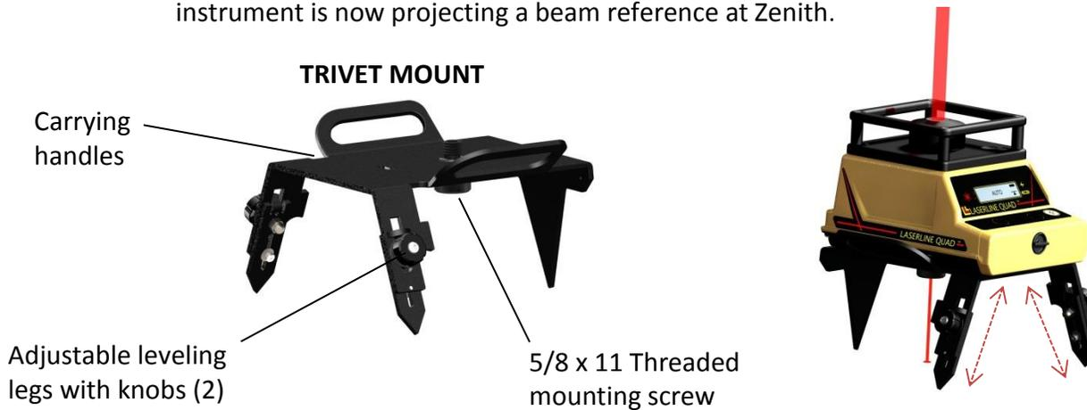
**USING A TRIPOD:** Standard flat head with 5/8 x 11 attachment
