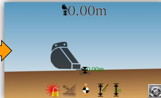
Same as when digging a horizontal reference, the screen and the LED display will indicate the actual difference of your bucket tip to the reference.
