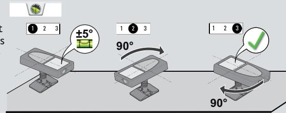
Rotate the device two times clockwise  $90^\circ$ . Follow the instructions on the display. Levelling is finished when OK icon appears on the display.
