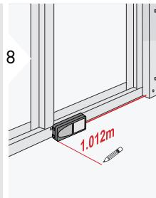
Move device slowly along the stake-out line. The distance to the next stake out point is displayed.
