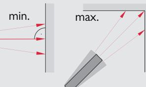
Used to measure room diagonals (maximum values) or horizontal distance (minimum values)
