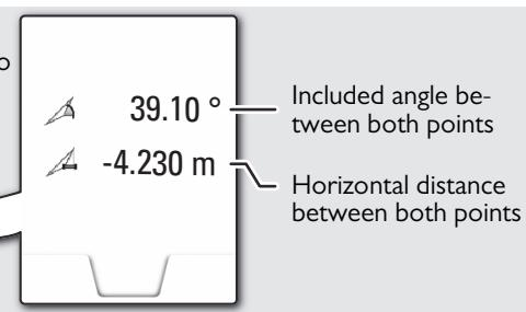
Indirect distance measuring between 2 points with additional results. Ideal for applications such as length and slope of roof, height of chimneys,...
