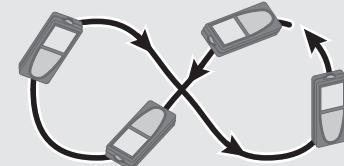
Rotate the device slowly in a figure 8 motion until OK icon appears on the display.
