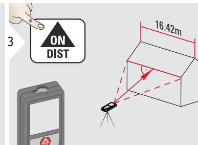
**It is absolutely necessary to aim with the laser perpendicular to the object.**
