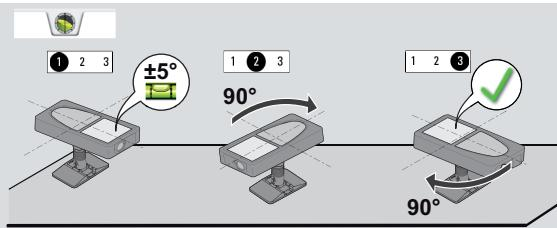
**Do not move device after levelling!**
