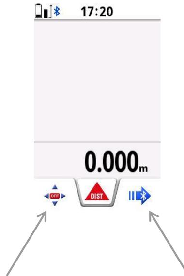
If switched on the Arrow keys on the DISTO™ can be used for navigation on e.g. Excel
