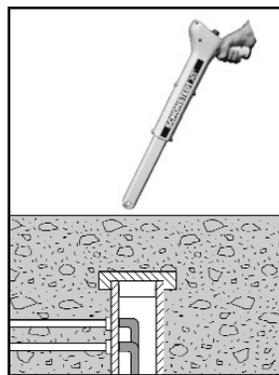
Figure 13. Locating Water Well Casings
