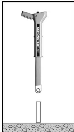
Figure 11. Checking a Stake's Orientation
