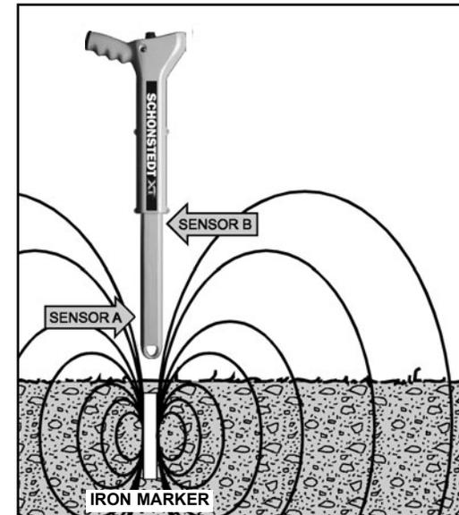
Figure 1. Detecting Magnetic Field of an Iron Marker
