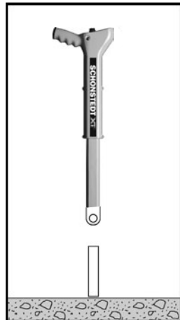
Figure 11. Checking a Stake's Orientation
