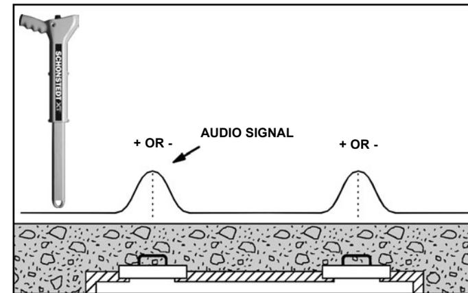
Figure 14. Signal Patterns Provided by Septic Tank Covers
