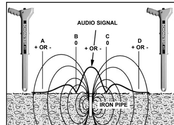
Figure 10. Signal Pattern from a Strongly Magnetized Marker
