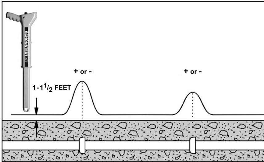
Figure 20. Signal Patterns Provided by Cast-Iron Pipes
