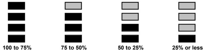
Figure 4. Battery Voltage Status Indications
