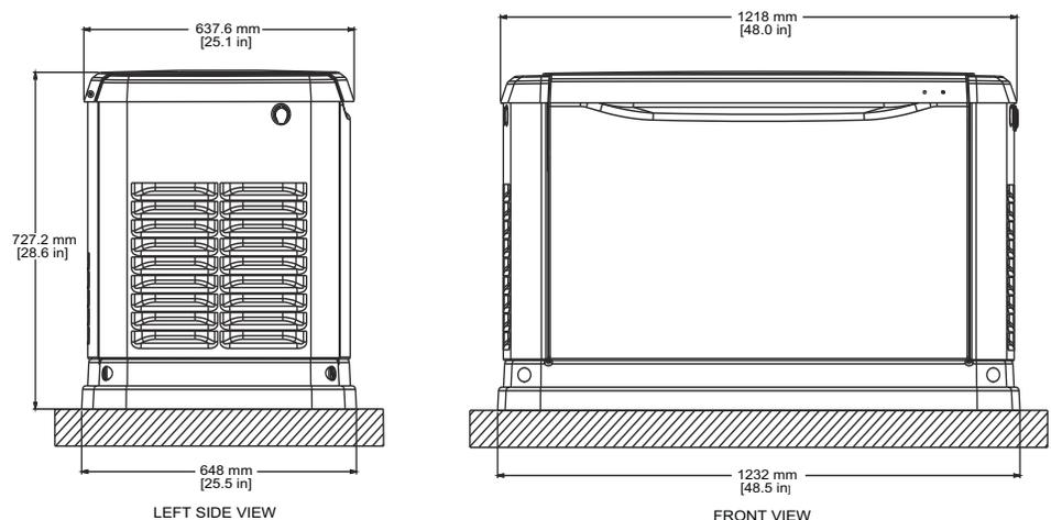
Dimensions shown are approximate. See installation manual for exact dimensions. DO NOT USE THESE DIMENSIONS FOR INSTALLATION PURPOSES.
