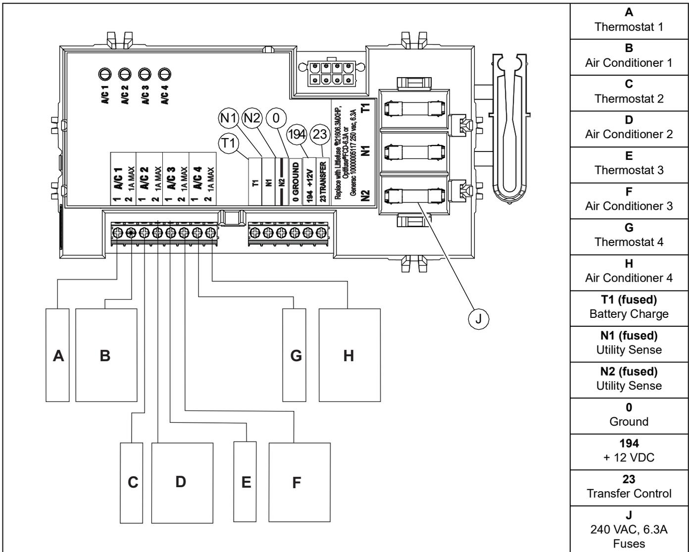
**Figure 3-6. Typical SACM Connections**
